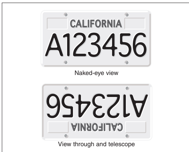
Figure 10. The view through a reflector telescope is upside down.
