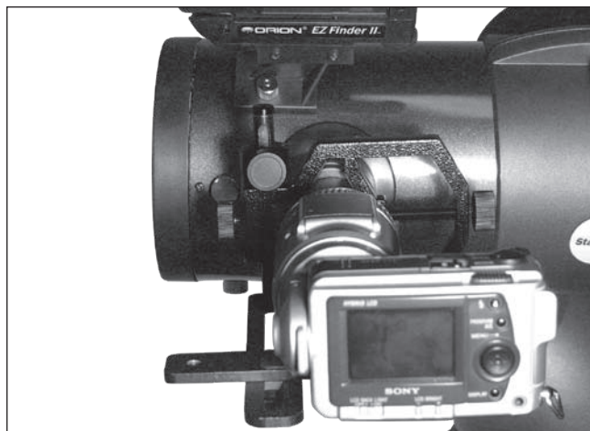
Figure 5. A camera attached to the SteadyPix Deluxe mounted on a reflector telescope and ready to use.
