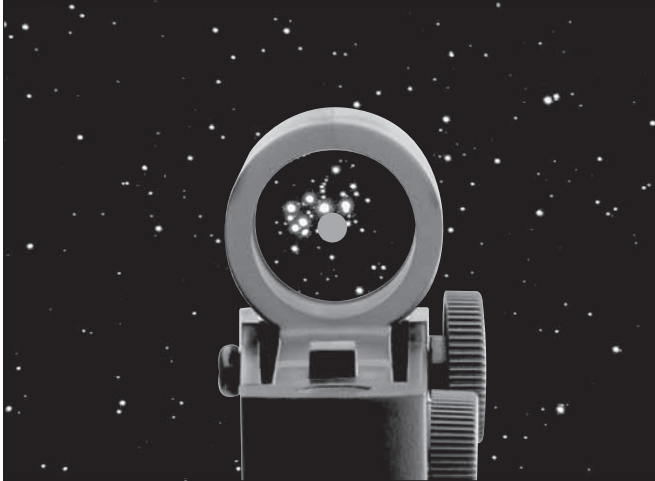
Figure 3. The EZ Finder II superimposes a tiny red dot on the sky, showing right where the telescope is aimed.
