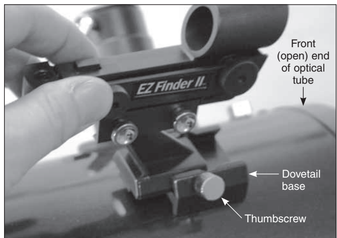
Figure 2. Insert the EZ Finder II in its dovetail base in the orientation shown and secure it with the thumbscrew.
