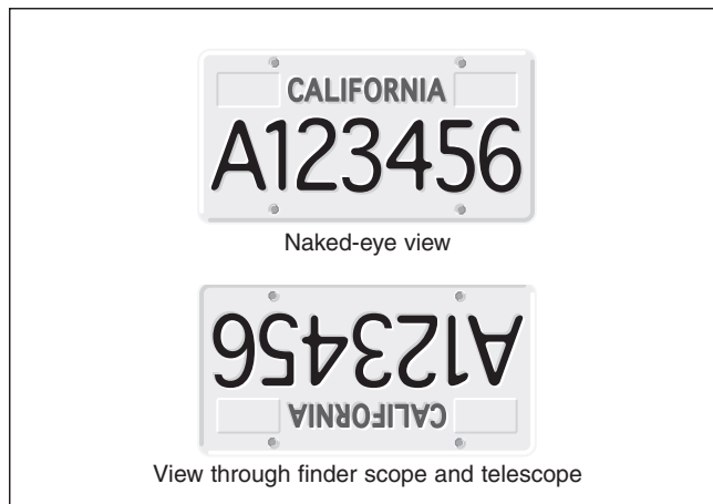
Figure 44. The view through a straight finder scope (and a reflector telescope) is rotated 180°.
