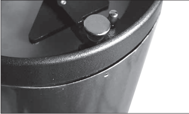
Figure 21. Locate the area of tube that is bulging out and preventing it from seating in the end ring. Press on the bulge to force the tube into the end ring.
