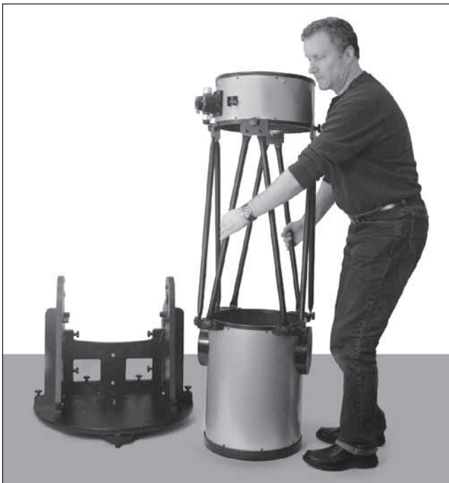
Figure 28. Lift the optical tube by grasping two truss poles and carefully lower it so that the large altitude bearing hubs rest on the altitude bearing cylinders on the side panels.
