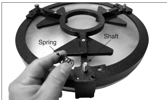
Figure 17. Place the three springs on the exposed threaded shafts of the mirror cell.
