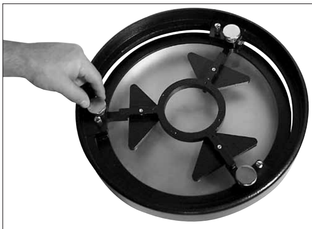
Figure 36. The tilt of the primary mirror is adjusted by turning one or more of the three collimation knobs.
