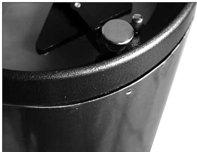
Figure 20. Locate the area of tube that is bulging out and preventing the end ring from fully seating.
