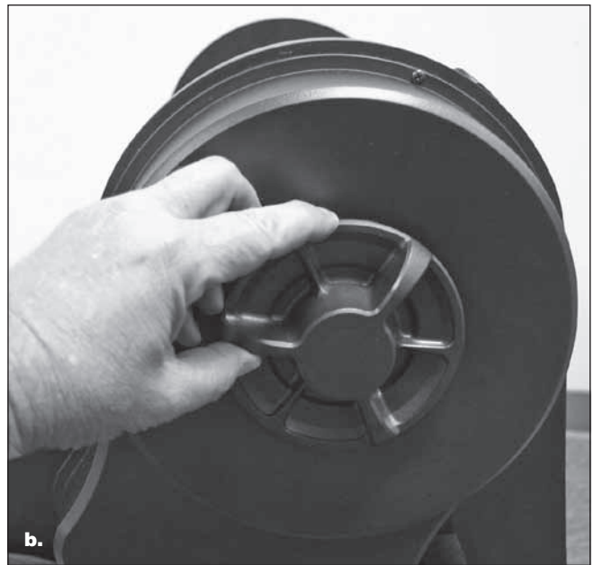
Figure 34. a) The redesigned altitude (Alt) and (AZ) azimuth motor/encoder housings of the XXg Dobs feature large manual clutch knobs for adjustable motion tension. b) Rotate the clutch knob to adjust the friction of motion for slewing the telescope by hand.
