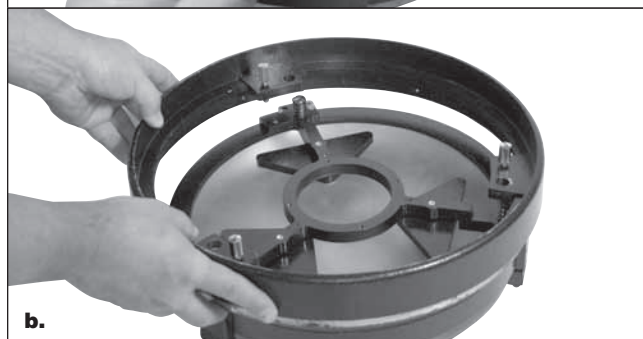
Figure 14. To remove the rear end ring, unthread the screws that connect it to the tube.
