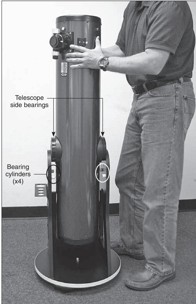
Figure 8. Gently set the telescope into the base by resting the side bearings of the telescope on the bearing cylinders.
