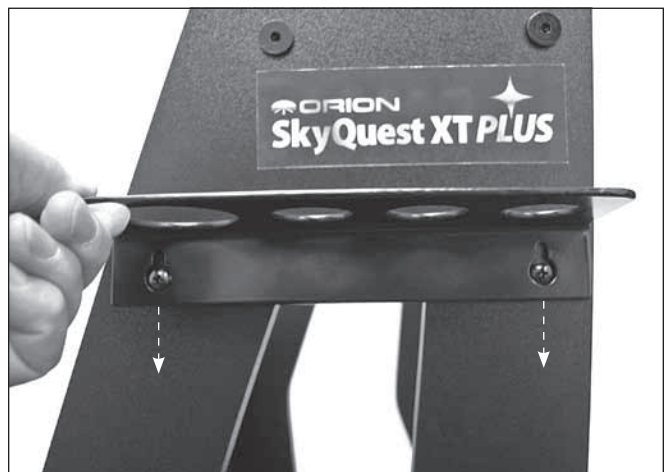
Figure 7. Place the eyepiece rack's "keyholes" over the mounting screws, then press the rack downward and tighten the screws. (XT8 PLUS rack shown)
