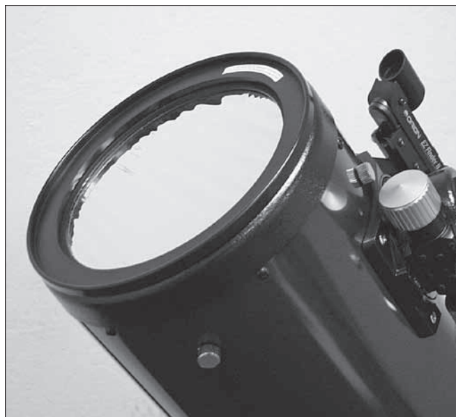
Figure 20. The included Safety Film Solar Filter snaps onto the front of the telescope for safe viewing of our Sun through the telescope eyepiece. DO NOT look through the EZ Finder II to center the Sun in the telescope's field of view!
