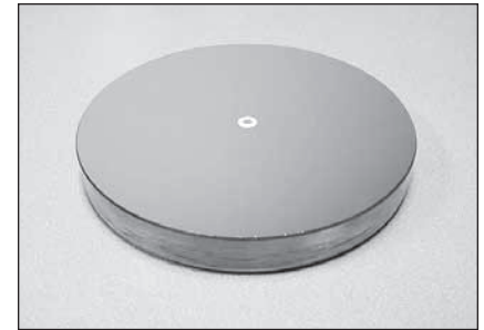
Figure 2. A center mark (ring) on a reflector's primary mirror greatly aids in collimation.
