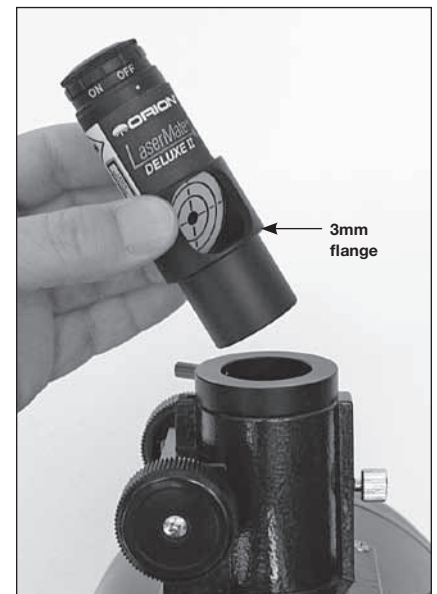
Figure 3. Insert the LaserMate's 1.25" barrel into the eyepiece holder of your focuser as far as it will go. It should seat squarely on the 3mm flange at the interface of the barrel and the wide section of the collimator's housing.
