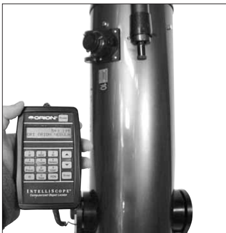
Figure 10. If you stand to the left of the telescope, and face the direction the tube is pointing, the guide arrows will correspond exactly with the direction you should move the telescope in order to find the selected object.
