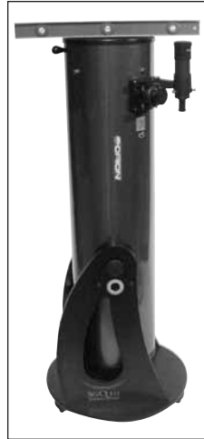
Figure 8. Place a carpenter's level on the base as shown. The base should stay level through a 180° rotation in azimuth. Once the vertical stop is set, the base does not need to be level to function properly.
