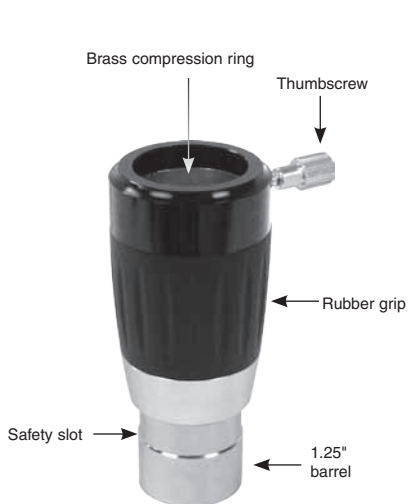
Figure 3. Mechanical features of High-Power Barlows (shown for a 1.25" Barlow)
