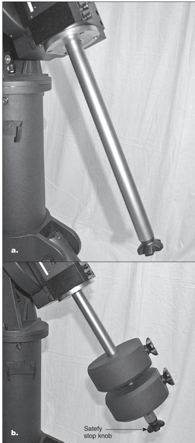
Figure 13. (a) The counterweight shaft threads into the mount. (b) Install the counterweight(s) and replace the safety stop knob.
