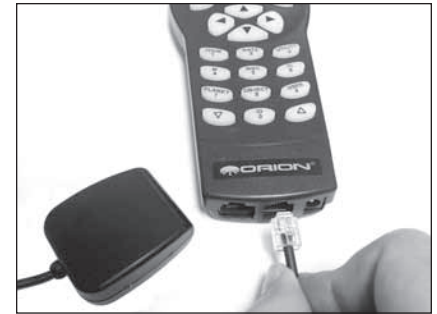
Figure 2. Connecting the GPS to hand controller.
