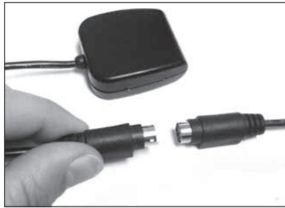
Figure 1. Connecting the GPS to the adapter cable.
