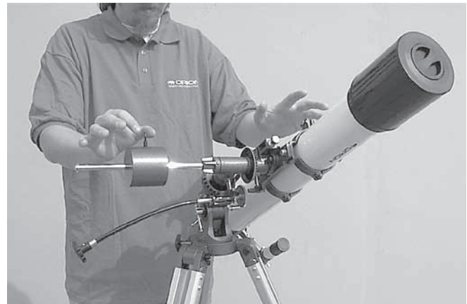
Figure 3b. Telescope is now balanced on the R.A. axis. That is, when hands are released, counterweight shaft remains horizontal.
