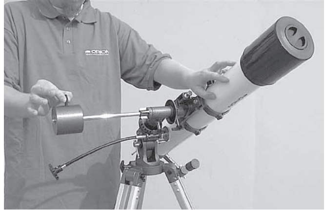
Figure 3a. Balancing the telescope with respect to the R.A. axis by sliding the counterweight along its shaft.
