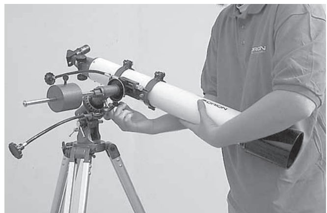
Figure 3c. Preparing the telescope to be balanced on the Dec. axis by first releasing the Dec. lock knob.
