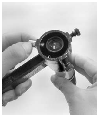
Figure 2b. Inserting the finder scope into the finder scope bracket
