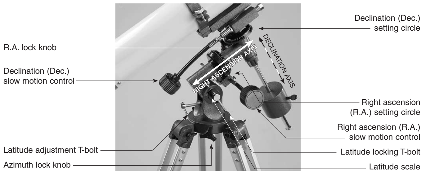
Figure 4. The equatorial mount.
