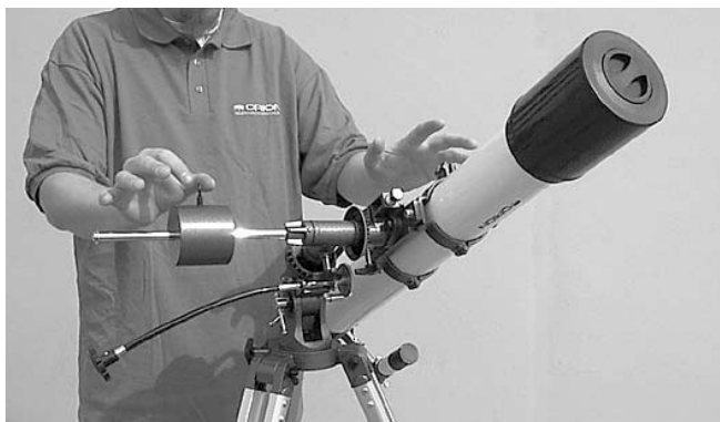
Figure 3b. The telescope is now balanced on the R.A. axis, i.e., when hands are released, the counterweight shaft remains horizontal
