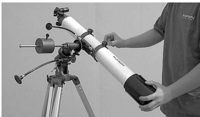
Figure 3d. Balancing the telescope with respect to the Dec. axis. As shown here, the telescope is out of balance (tilting).
