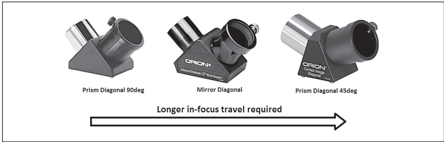
Figure 3. If more in-focus travel is required a 90 degree Prism Diagonal may be required. A 45 degree Prism Diagonal requires more in-focus than any other diagonal.
