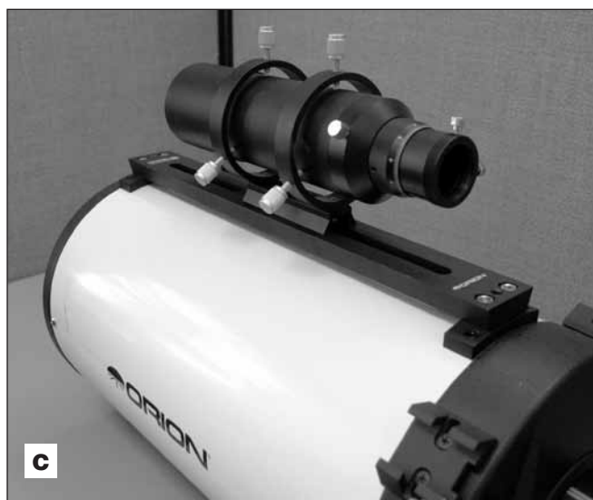
Figure 3. A) The bracket's dovetail bar has one 1/4"-20 (center) and two M8x1.25 threaded holes for attachment to an optional universal dovetail plate (B). In C) the guidescope is mounted on the top plate of an Orion 8" Ritchey-Chretien telescope.
