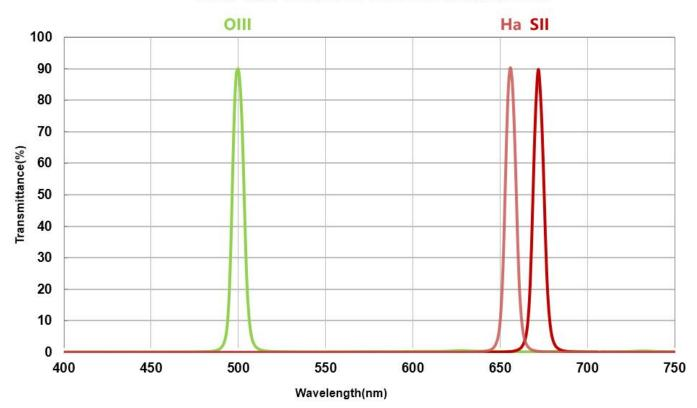
The new OIII filter is based on the same base glass, with a new coating standard and better block rate of off-band.
