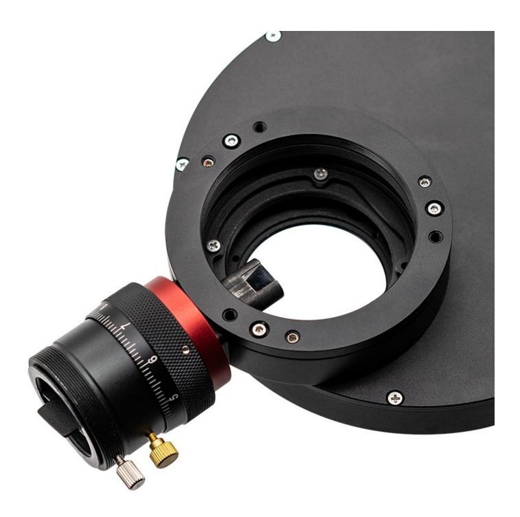
The original M54 sensor tilt plate of ASI6200 can only be used to connect with the M42/M48 thread telescope side for now. While this new M68 sensor tilter plate can be used to connect with the M68 thread telescope side.
