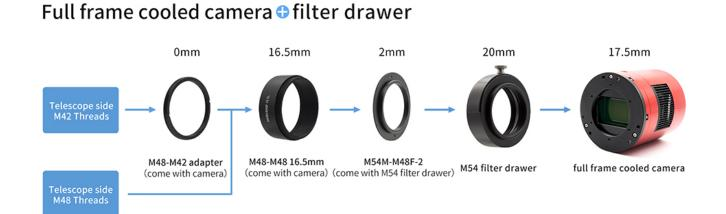
Note: This solution can only reach 56mm back focus length. If you want 55mm back focus length. Also the M48-M42 adapter will block the camera sensor a little bit. So we recommend you use 2"EFW with M68 OAG
