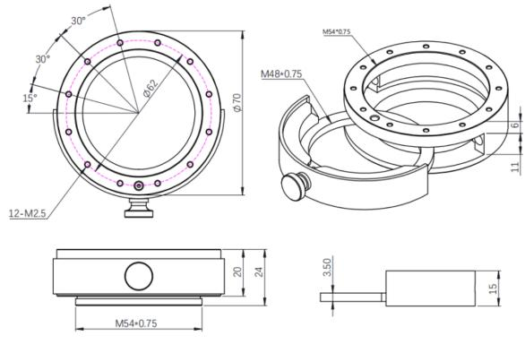
70mm(height)\*70mm(length)\*20mm(thickness) M54\*0.75 male(external) thread (camera side) M48\*0.75 female(internal) thread (filter end) M54\*0.75 female(internal) thread (telescope side) Suitable for 2-inch astronomical filters
