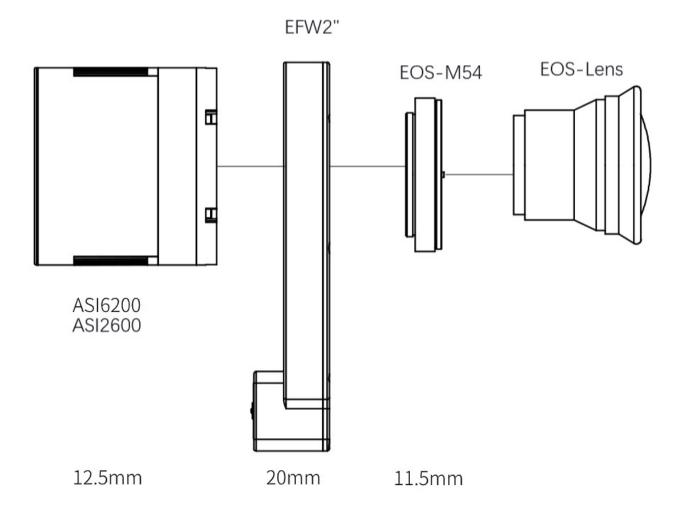
Note: The sensor tilt adapter needs to be removed before you mount the camera with the 2" EFW.
