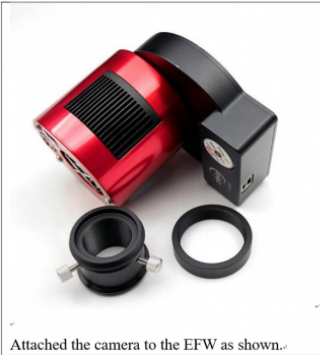
Take out the 1.25" T-Mount form the T2-1.25" holder.
