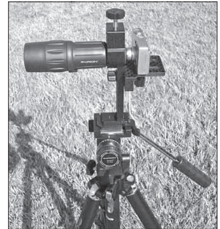
Figure 8. The SteadyPix Pro is shown attached to a photo tripod via the 1/4"-20 socket in the SteadyPix's foot. A monocular is held in the eyepiece clamp.
