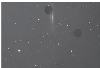
Figure 15.2. Dust or other particles on the camera's optical window can show up as distracting dark shapes in your images.
