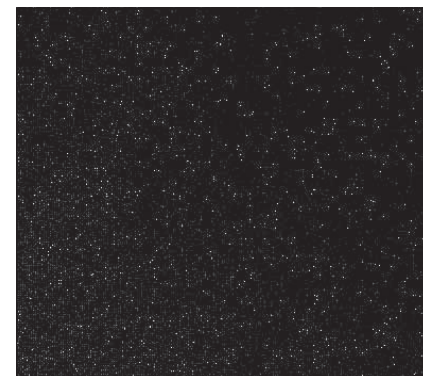
Figure 14. A dark frame contains the thermal and background noise, as well as any read noise. The same noise appears in your "light" images. Dark frames isolate the noise so it can later be subtracted from your "light" images.
