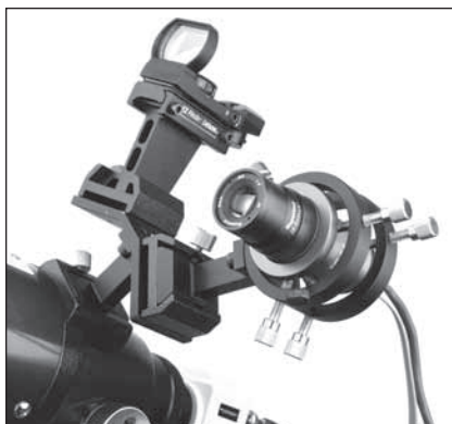
Figure 19: The SSAIO configured as a digital finder.
