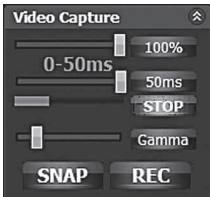
Figure 5: The video Capture interface showing Gain, Exposure and Gamma settings.
