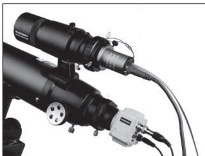
Figure 21. The SSAIO setup for guiding using the Orion Mini guider with helical focuser.
