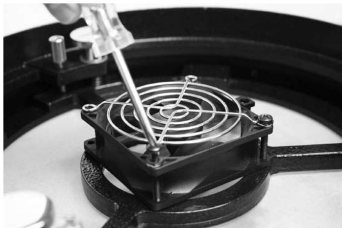
Figure 2. Attaching the fan to the mirror cell.
