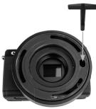
**2. FOR SONY CAMERAS:** Use the tip of the tool to depress the camera's lens release button, then rotate the adapter counter-clockwise.
